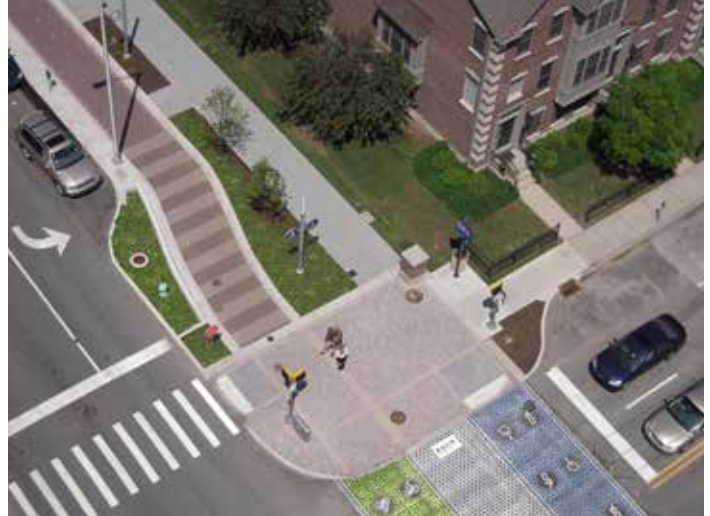
Image: Example a widening of sidewalk, providing curb extensions and bike lanes to create a safer neighborhood street. (Source: Visit Charlottesville)
